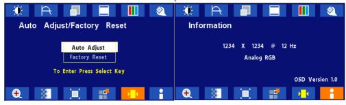
Push the select button to execute the Auto Setup function or Push the select button to execute Recall Factory Default
